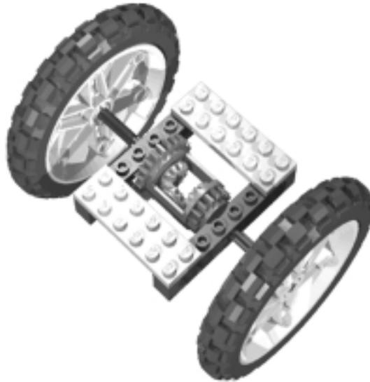
To use this configuration in a vehicle, you simply have to apply power to the body of the differential gear, which incorporates a 24t on one side and a 16t on the other.
