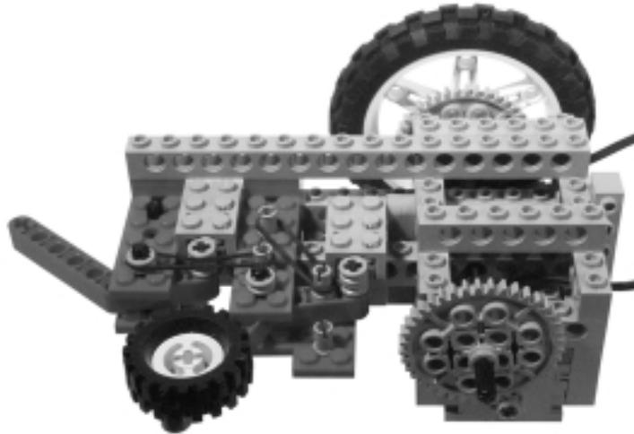
Our robot is very low to the ground because we placed the motors below the beams that support the wheels, but in this kind of task we don't need a lot of ground clearance and this solution keeps the assembly nicely compact (Figure 19.8).
