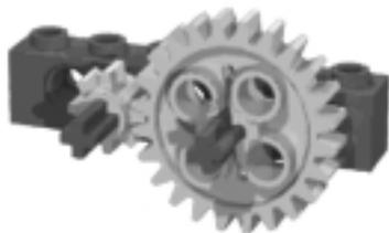
Let's go back to our example. We have two gears, an 8t and a 24t, each mounted on an axle. The two axles fit inside holes in a beam at a distance of two holes (one empty hole in between). Now, hold the beam in one hand, and with the other hand gently turn one of the axles. The first thing you should notice is
