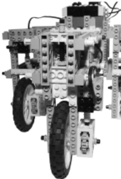
The RCX stays on the top, just behind the point where the bogies connect to the body (see Figure 16.11).
