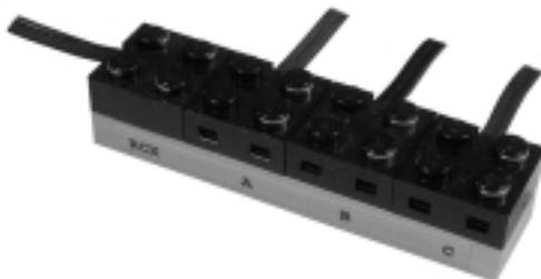
Nitin Patil designed a more complex multiplexer suitable for connecting a single input port to three active sensors, like the original light and rotation sensors, or any other custom active sensor like IRPDs, sound, and so on. Active sensors use
