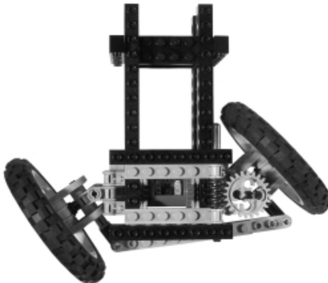
Notice also that the arm connecting the wheels does not remain parallel to the front side of the chassis. For this reason, it's not possible to employ the simple rack and pinion scheme we used before. You should substitute the jointed arm for
