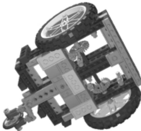
You can also remove the pivoting wheel and the two main wheels in a matter of seconds to reuse them for another project (Figure 5.10). We should mention here that the pivoting wheel is quite special, since it's what makes a two-wheeled robot stable and capable of smooth turns. The technique of making a good pivoting wheel has its own design challenges, of course, which we'll explore in Chapter 8.
