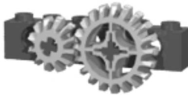
Things get a bit more complicated when you want to couple two of the same kind, as the resulting distance is 1.5 or 2.5. And even more complicated when combined with other gears, causing resulting distances that include a quarter or three quarters of a stud. These gears are designed to work well in perpendicular setups as well (Figure 2.15).
