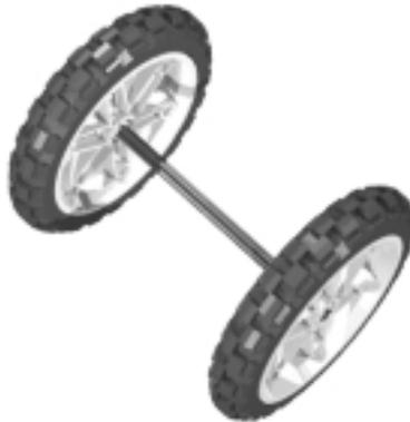
The reason is that when two parallel wheels turn, their paths must have different lengths, the outer one having a longer distance to cover (Figure 2.21). In our example, in which the wheels are rigidly connected, at any turn they cover the same distance, so there's no way to make them turn unless you let one slip a bit.
