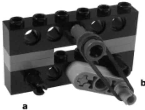
Applying this principle, we designed the pliers shown in Figure 11.5, which are suitable for grabbing very small objects like a 1 x 2 brick (seen at the bottom of the Figure between the two plates). To actually use them in a robot you must add a motor that, through brief impulses, pushes the pliers into their open or closed states. As usual, you would probably involve a belt or a clutch gear to make the timing of the motor not critical.
