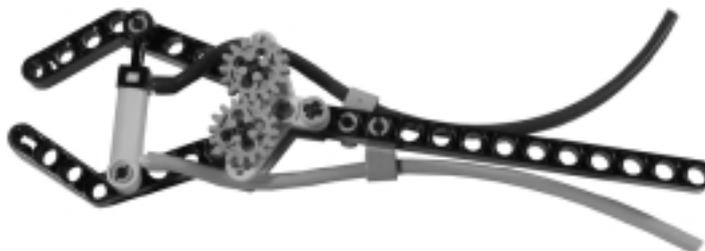
The flex system we briefly described in Chapter 9 has similar properties, allowing you to transfer motion to distant parts. Our robot, Cinque, features a small operating hand based on this technique (see Figure 11.8). A pair of opposing rubber bands introduce a degree of elasticity into the system, and help the fingers return to their default setting once the hand comes to rest in its open position.
