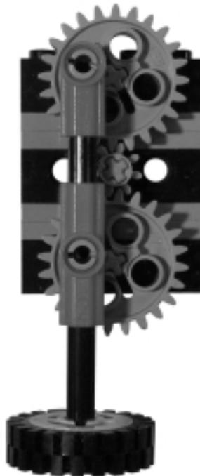
By driving any of the three gears, this simple leg will go up and down, forward and back, always in a circle. The leg always remains vertical. Figure 15.13 shows a slightly different approach, where only one point of the leg is attached to the wheel, and the leg itself slides freely into a rotating support (fulcrum).
