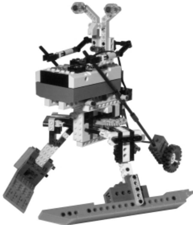
To build the skis you need some extra beams and, more important, many tiles (see Figure 16.14). We used 36 2 x 2 and two 1 x 4 tiles (available as spare parts at the LEGO Online Shop). If you are open to employing non-LEGO parts, you can build the skis from other materials, like strips of plastic available in hobby shops.
