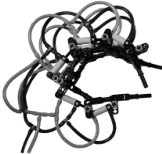
The degrees of freedom concept applies not only to hands but to any mechanical device. The arm of Figure 11.12, taken from our R2-D2 styled robot “Otto,” has two degrees of freedom: A large cylinder extends the arm from the body of the robot, and a small one operates the hand.
