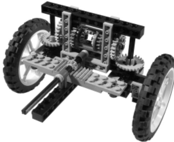
The trick we used here is to send the motion to the wheels along their pivoting axles, exactly like in a synchro drive. And the wheel assembly also works like the one used for our synchro of Chapter 8 (Figure 14.24).
