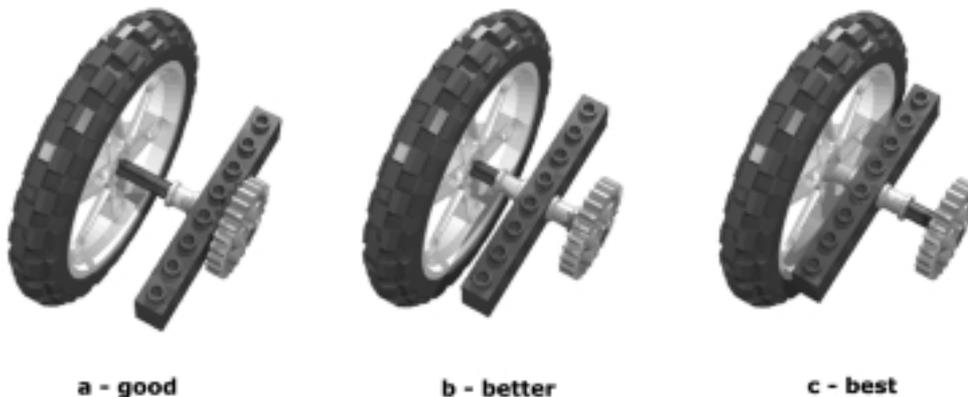
We suggest you also support the load-bearing axles with more than a single beam whenever possible. The three examples shown in Figure 5.6 are better than those in Figure 5.5, with 5.6c being the best among all the solutions shown so far. The use of two supports, one on either side of the wheel, like on a bicycle, avoids any lever-effect created by the axle on the support, thus reducing the friction to a minimum.
