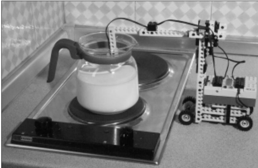
The chassis has no turning ability at all, as this robot doesn't need it (Figure 25.7). The gear ratio is 1:9, obtained from two 1:3 stages. Together with the small wheel diameter, this ratio makes the robot very slow. There's no particular reason for such a geared down configuration, except that the robot is not in a hurry, and that there are all those nice gears in the MINDSTORMS box that would be a pity to leave unused!
