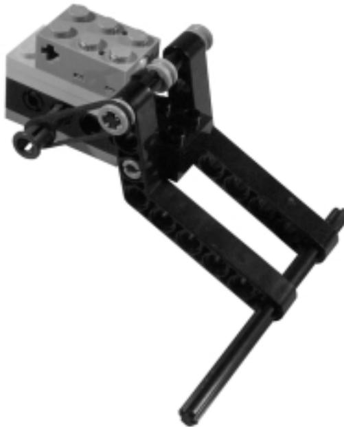
**Figure 14.4** The Robot, Complete with RCX and Bumpers
