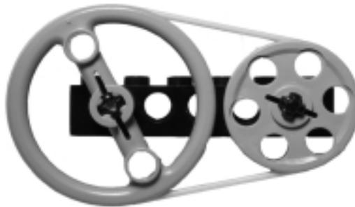
You must also consider that pulleys are not very suitable to transmitting high torque, because the belts tend to slip. The amount of slippage is not easy to estimate, as it depends on many factors, including the torque and speed, the tension of the belt, the friction between the belt and the pulley, and the elasticity of the belt.
