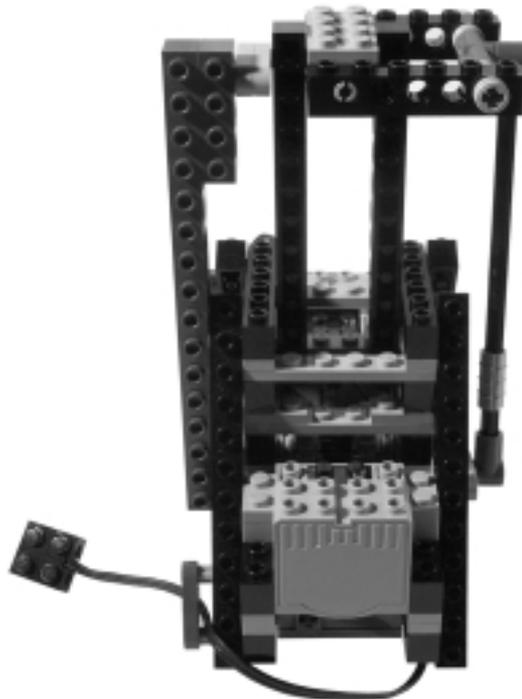
Those long arms are linked to liftarms, each one mounted on an axle that goes right in the middle of the assembly and ends on a 24t gear (Figures 24.10 and 24.11). The two diagonal beams that lock the assembly are not a perfect match: They form a triangle with sides 4 and 8, which correspond to a hypotenuse of about 8.94 instead of the 9 we used. This small difference—less than seven parts per thousand—is close enough for a solid connection.
