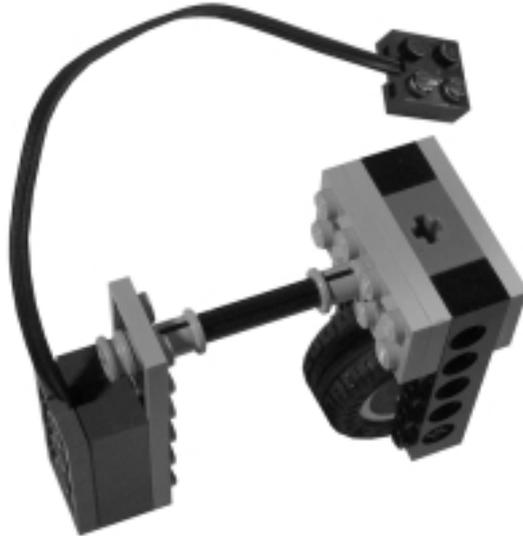
Notice that we used the indented side of the bushings to attach the axle to the plates: It perfectly matches the area among the four studs, and its friction is enough to allow the axle to carry a small weight.
