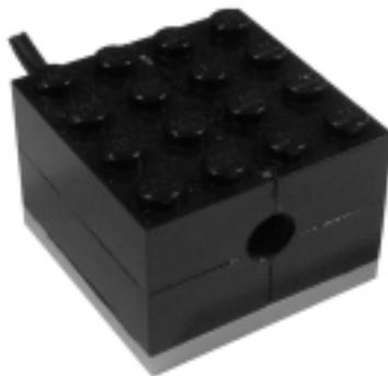
The casing around the pyroelectric sensor has a small hole that lets its internal “eye” receive the infrared light any warm body produces. It requires some time to adapt to the ambient radiation, but afterward it can detect any change in intensity. These features make it unsuitable for mobile robots, but it’s very useful in those projects where a robot must start doing something when it detects a human presence.
