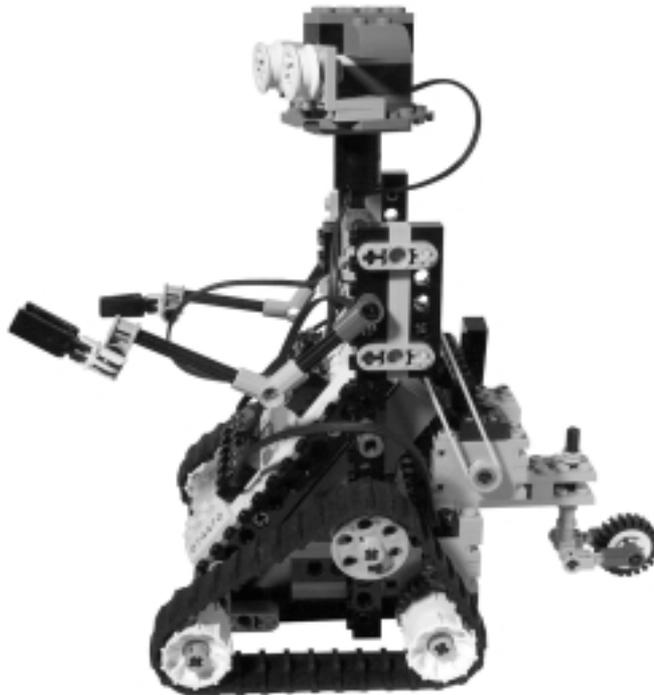
The gearing of the drive motors is rather simple: an 8t gear on the motor shaft engages a 24t gear connected to the drive axles. (Remember that you also need a 16t gear inside the track wheel to joint it to the axle.)
