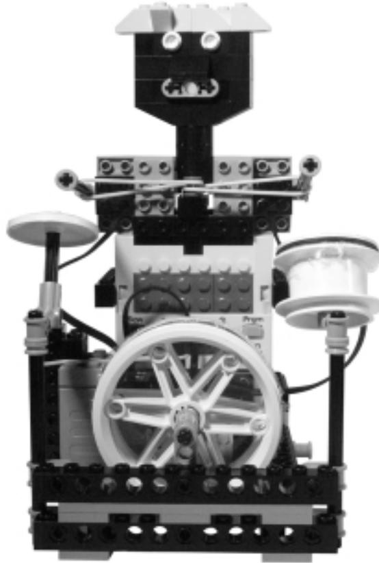
Two 16 long beams run vertically across the back of the robot, supporting the motors and the RCX (Figure 21.5).
