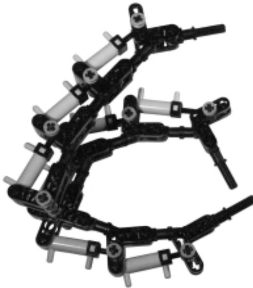
**Figure 11.11** The Three-Finger Pneumatic Hand with Complete Tubing
