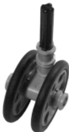
The casters shown in Figure 8.6 get much better results. The one on the left uses a single wheel, thus avoiding the problem entirely. The one on the right, which is more solid, uses two free wheels that allow the caster to turn in place without friction or slippage problems. The difference is in the wheel hubs. In the assembly on the left, the axle turns with the wheel, while the one on the right has the wheels spinning on the axle.
