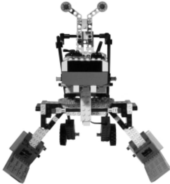
**Figure 16.16** Alternative Leg Geometry
