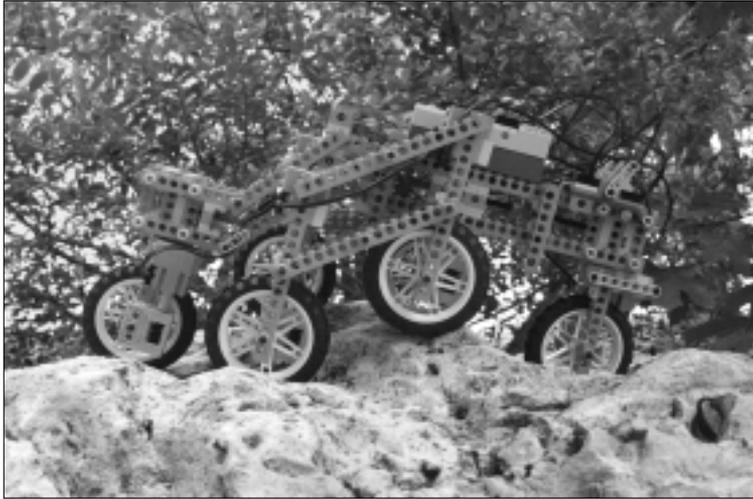
In our turning SHRIMP, we adopted a simplified scheme: the front and rear wheels turn, while the bogie wheels behave like a skid-steer. In other words, the inner ones stop while the outer ones continue to run. This is an approximate solution that introduces some slippage, but that in practice works very well on most terrains.
