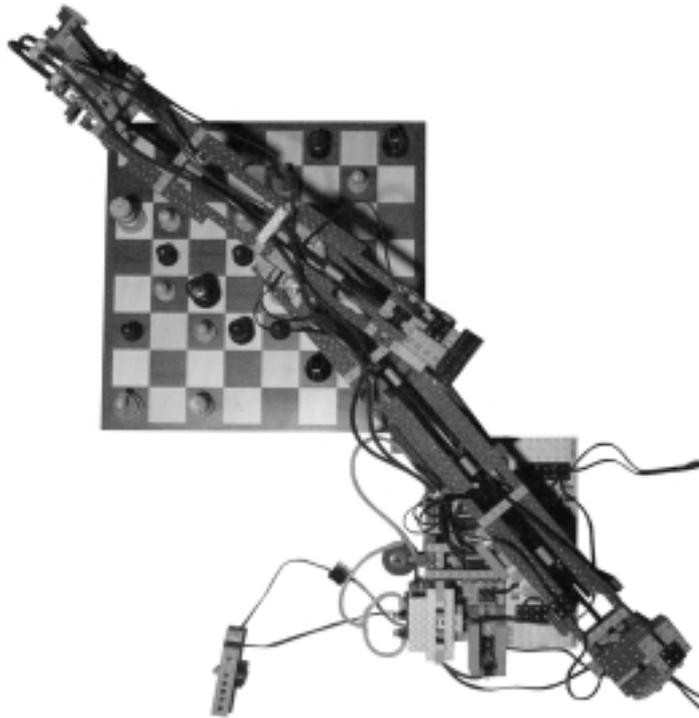
We used a rack and pinion assembly for the lifting mechanism, and a small pneumatic cylinder for the pliers (Figure 20.7).
