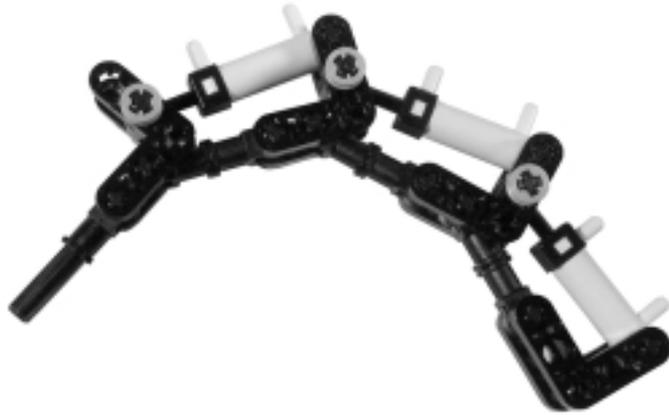
**Figure 11.10** A Three-Finger Pneumatic Hand
