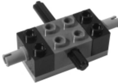
This jointed chassis connects to two arms that operate the pitch and bank movements. The front one adjusts pitch, while the rear one changes bank (Figure 24.9).
