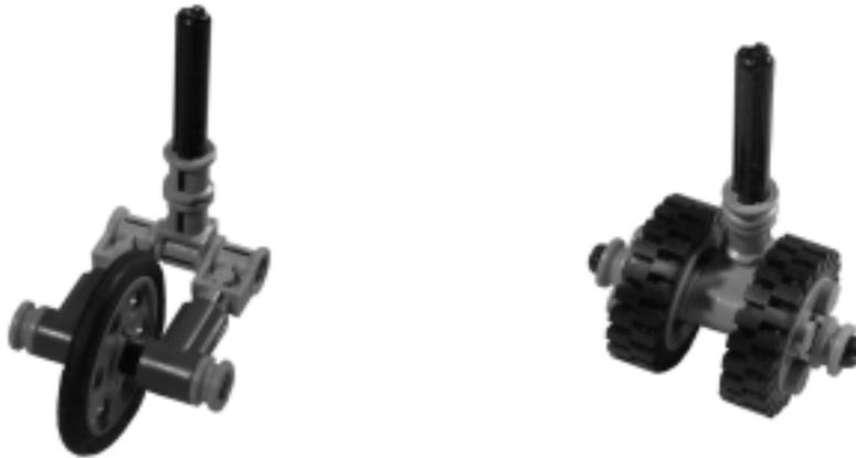
The choice of using one or more casters depends on what task the robot is designed for. A single caster is enough for most applications, but two casters at the front and rear of the robot are a better option when stability is important.
