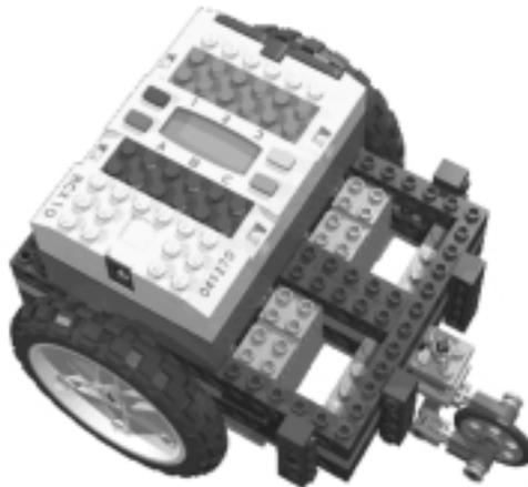
As you move the RCX toward the pivoting wheel, the robot becomes more stable (Figure 5.12). It still jumps a bit on sudden starts and stops, but it doesn't flip over anymore.
