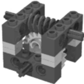
Another fact you have likely observed is that the two axles are perpendicular to each other. This change of orientation is unavoidable when using worm gears.
