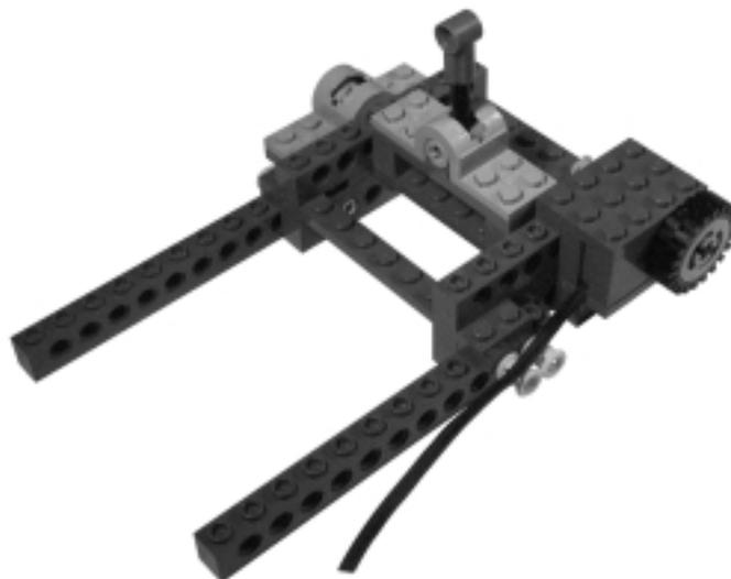
There are six long wires that run from the remote to the platform: two from output ports A and B to the motors of the differential drive, two from input ports 1 and 2 to the rotation sensors for pitch and bank, and two from the polarity switches to the pitch and bank motors. The throttle rotation sensor connects directly to input port 3, and you need two more short cables to bring power from output port C to the polarity switches.
