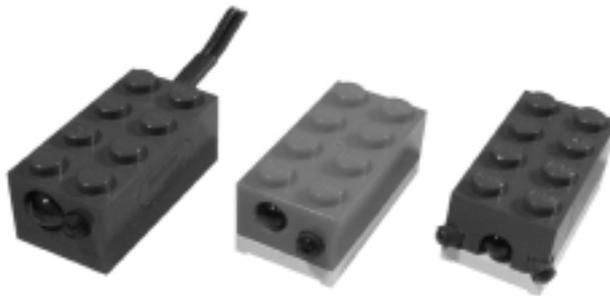
Sevick also produces a *pitch sensor*, a sophisticated sound sensor that returns a value proportional to the frequency of the incoming sound. You can thus control your robot by simply whistling or playing a flute or recorder like a modern Pied Piper. The robotic pianist of Chapter 21 represents a possible application for this sensor: It can learn a simple melody just by listening to it.
