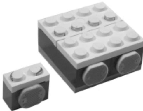
Recycling junk is an option when trying to save money. Figure 9.11 shows a touch sensor made with a switch from a computer mouse. Pulling apart a broken mouse, you will discover that there are some micro-switches connected to its push-buttons. Unsolder them from their circuit plate, solder their terminal to an electric plate, then add some parts to the case in the switch.
