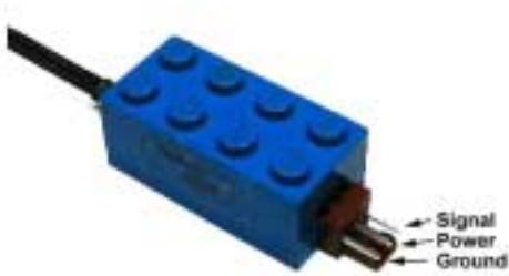
The converter brick has a Lego bump connector that snaps directly on to your RCX. The other side of the converter has three pins: Power, Ground, and Signal.
