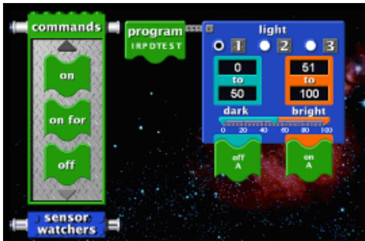
The program value is inversely proportional to the electrical signal. Five volts input is read as zero by the program. Zero volts in is read as 100 by the program. (Exactly backwards of what you might expect).
