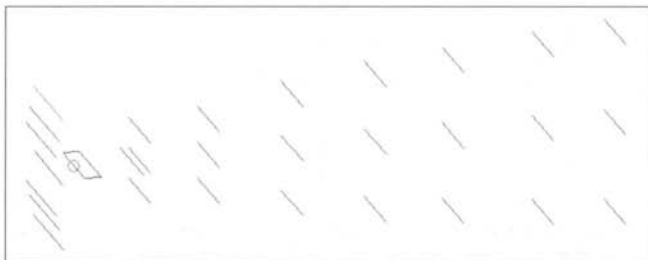
Fig. 1 Layout of the Fan Yagi Array (Tri-axle Yagi) optimised using Genetic Algorithm technology
