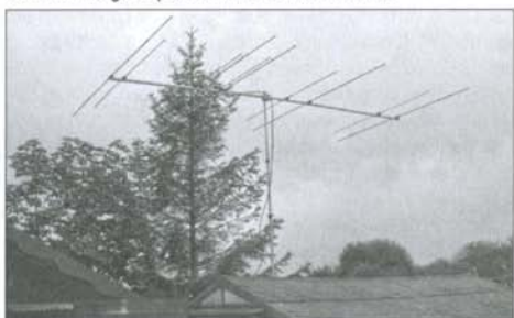
YU7EF design 5 + 5 ele duo band yagi for 6m and 4m using a single feed @ G7CNF
