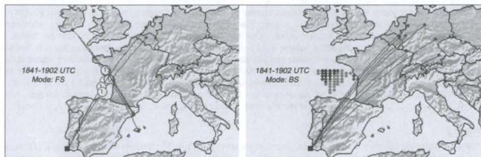
Fig. 0.4. Phase 4 of the June 5, 2007 event showing a mixture of sporadic E forward (left) and backscatter (right) communication links. The radio contacts on the right hand side represent the longest communication distances (along the great circle) in sporadic E backscatter ever observed in Europe.
