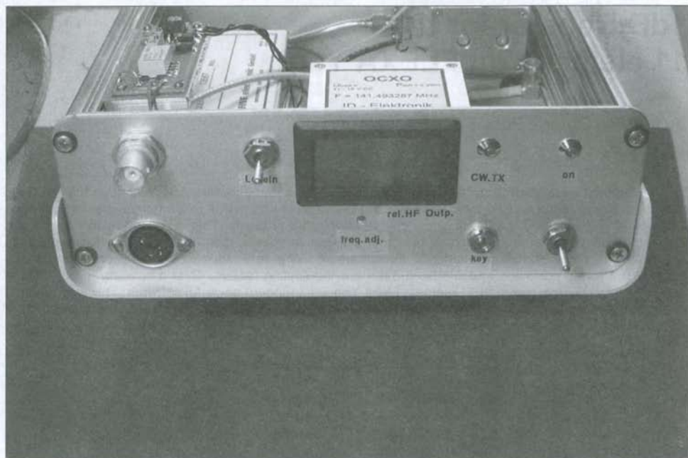
Picture 20 - 122 GHz beacon TX with LC readout
