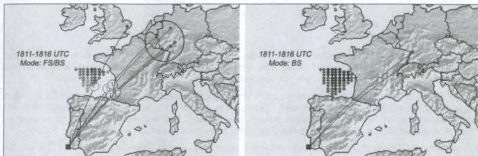
Fig. 0.2. Phase 2 of the June 5, 2007 event which has enabled forward- (left) and backscatter (right) radio contacts. The lines represent the great circle paths between the actual transmitter and receiver. Note that the great circle paths are identical to the radiowaves' propagation path in forward scatter but are not identical to the radiowaves' propagation path in backscatter.
