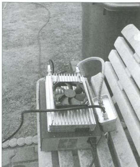
Amp and preamp are being placed as close as possible to the antenna – even if this means on a garden bench
