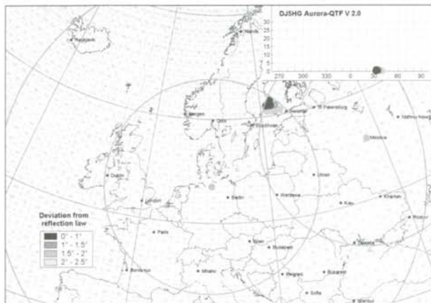
Fig 5. Illustration of all possible scattering points for aurora communication between Hamburg and Moscow. Please note that only QTF 32° is possible. A high-gain, narrow-beam antenna is optimum for this case.
