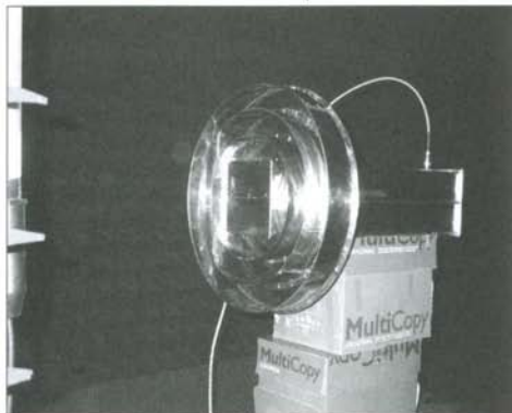
OM6AA's Modified Septum Feed in anechoic chamber
