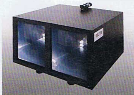
PHOTO 14: The 'big rig' with Fresnel lenses, suitable for a Tx and Rx or a transceiver and beacon (remove the lens on the beacon side).
