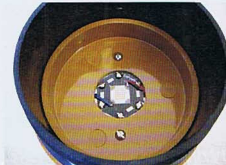
PHOTO 11: The extreme beacon LED mounted in one of our now-standard housings.
