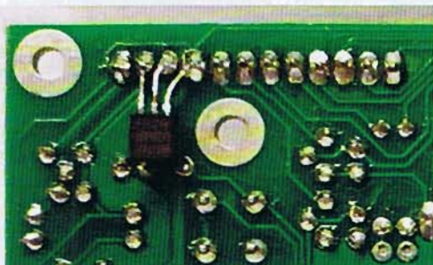
PHOTO 1: 5V regulator mod for G6ALU controller board.
