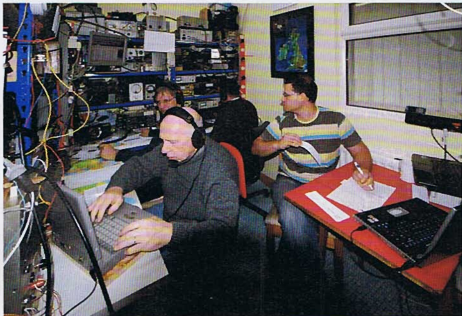
PHOTO 1: Five Bells contest group in the October contest. Left to right Paul, M0WAF working 1.3GHz, Keith, G4ODA, operates 2.3GHz new higher power masthead system for 2010, Paul, G1LSB, operates 432MHz (just used for the 8 hours of the Trophy contests to 'lift' contacts to 1.3 and 2.3GHz) whilst Howard, G0VTL operates KST to make skeds. Photo: Bob, G1ZJP/M1MHZ.
