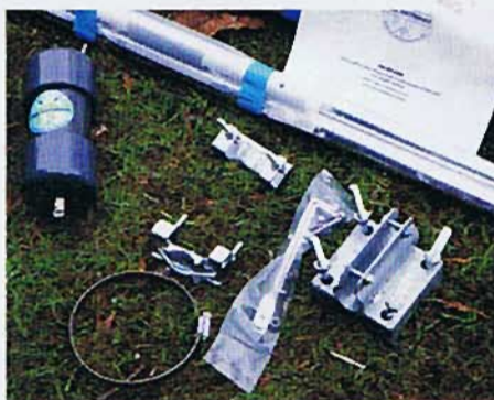
PHOTO 2: The balun and mounting hardware.
