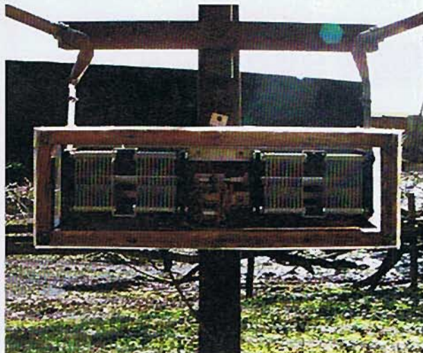
PHOTO 2: Detail of the tuning capacitance mechanism.
