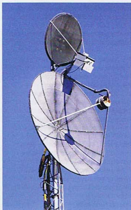
PHOTO 2: Antenna system belonging to OZ1FF. The 1.5m dish is shown with multiband feeds for 1.3, 2.3 and 5.7GHz. The smaller 65cm dish carries feeds for 10GHz and 24GHz. Photo: Kjeld, OZ1FF.
