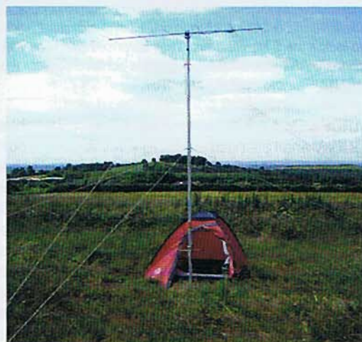
PHOTO 3: G4ARI/P's mast, antenna and accommodation.
