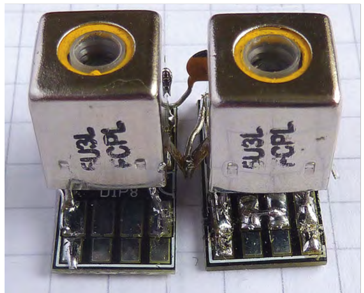
Small bits of p.c.b. material make suitable 'Manhattan' style mounting pads for 10k type coils.
