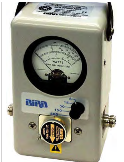
Probably the most well-known s.w.r. and power meter, the Bird Thru-line uses separate sensors for differing power levels and frequencies.
