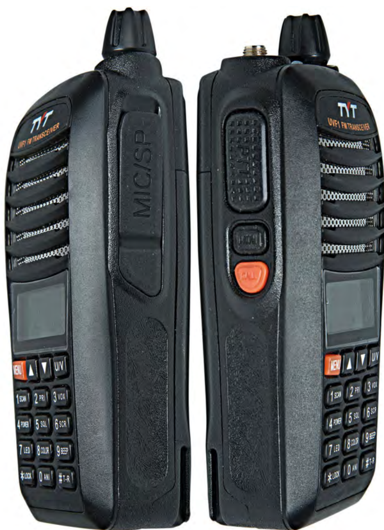
Two views of the sides of the rig, a dual coaxial socketed microphone connection is under the upper 'flap' on the side of the left hand rig.
