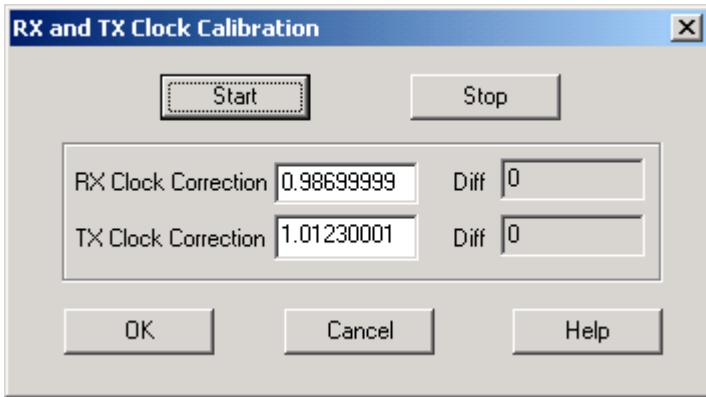
The calibration is started by clicking 'Start' button and stopped with 'Stop' button. The exact calibration values for RX and TX are shown in the separate window. The calibration routine should be run about 30 minutes. Finally click 'Ok' and the dialog will close and the values will be saved.
