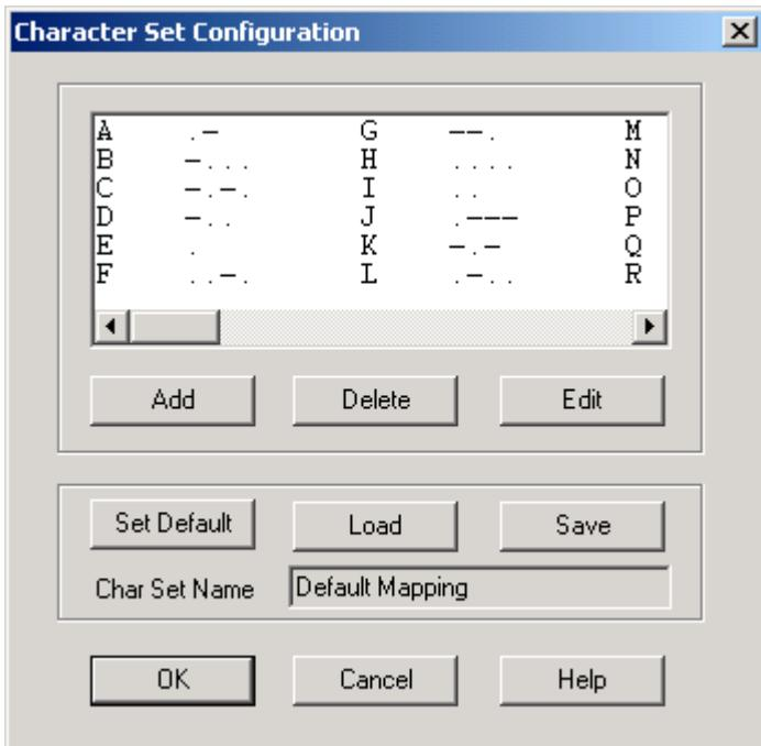
New characters can be added for CW by pressing the 'Add' button. In RTTY, the button is disabled, because the total amount of characters (=64) is fixed.
