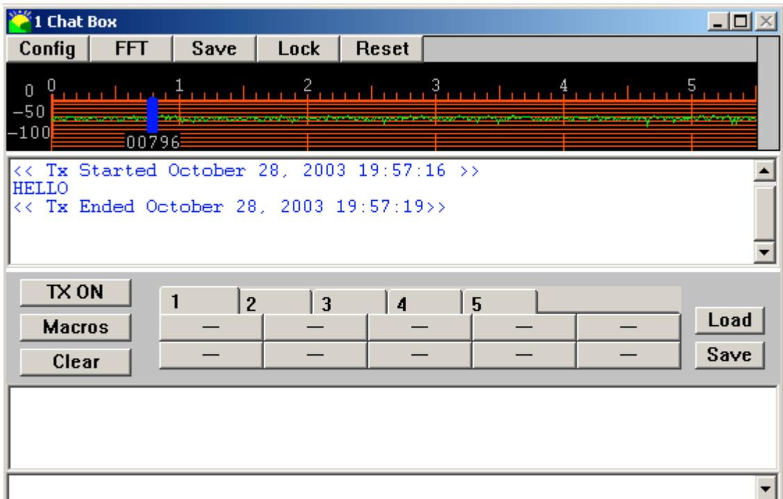
The upper window is called the RX window and the lower window is called the TX window. The TX window contains the [TX macro panel](#), which is used to copy predefined blocks of text into the TX window. The TX window contains also the TX edit line, where test can be written when transmitter is on. Pressing enter the line is copied at the end of TX transmitter
