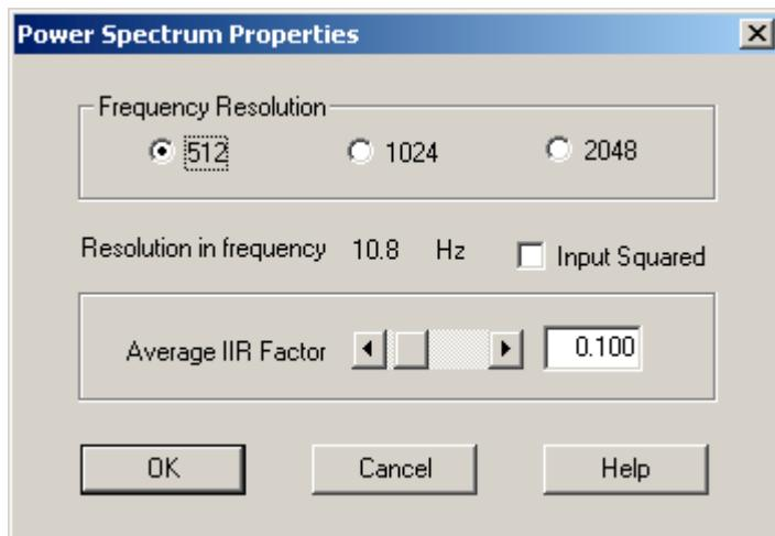
The resolution of the power spectrum display can be selected at 512, 1024 or 2048 samples. The bigger the value, the better is the resolution in the frequency domain. The resolution also depends on the sampling frequency. The average IIR factor parameter is used as the IIR gain factor in the averaging process. It is used only when the averaging mode is on. A smaller gain factor means that new values have less gain compared to the old values.
