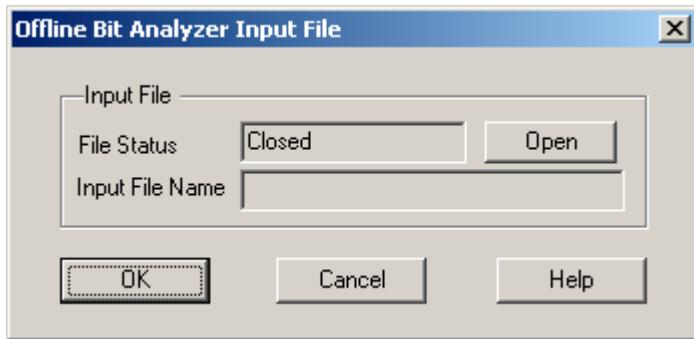
Press the ‘Open’ button to open bit log file. The file status shows if the file is already open and the input file name field gives the name of the bit log file.
