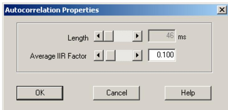
The length of autocorrelation can be selected with the horizontal scroll bar. The length of autocorrelation window is shown as milliseconds. The average IIR factor parameter is used as IIR gain factor in the averaging process. It is used only when averaging is on. A smaller gain factor means that new values have less gain compared to the old values.
