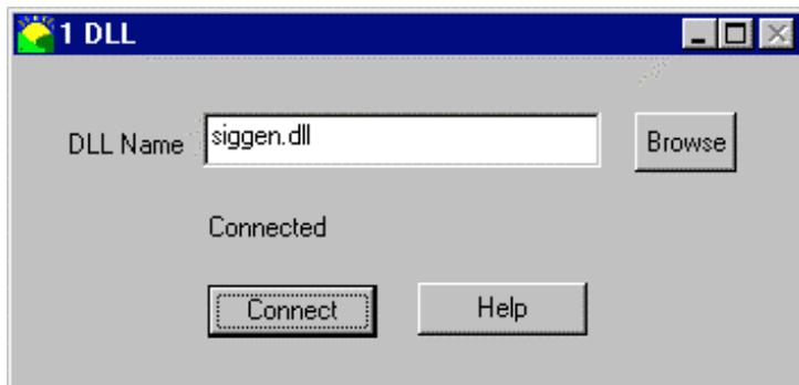
The DLL plug-in has to contain at least one routine called *Process*. SkySweeper calls the *Process* routine to pass data for processing. The routine contains two input parameters: InWaveHder and OutWaveHdr, which are the WAVEHDR (waveheader) structures. The WAVEHDR structure defines the header used to identify a waveform-audio buffer, and it is defined in the file called mmsystem.h. The data is in the floating point format.
