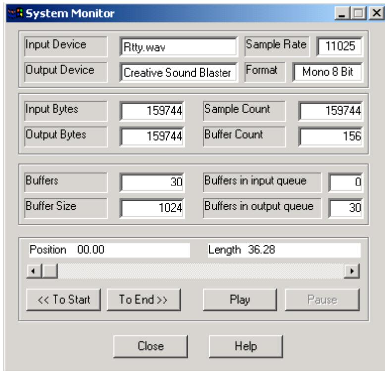
The dialog shows which input and output devices are selected and their sample rates and formats.
