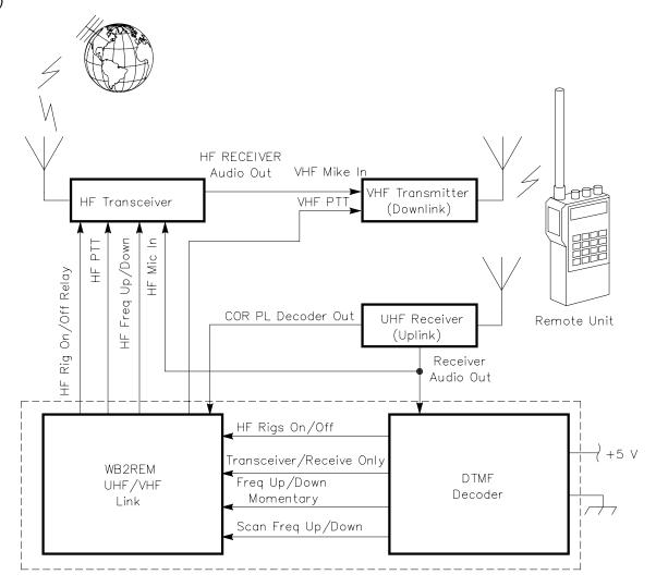
Figure 1—A block diagram of WB2REM's remote link.
