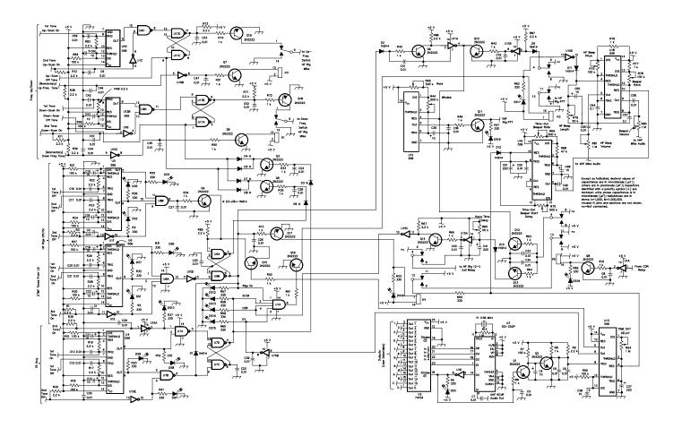
Figure 2—Schematic of the WB2REM remote link. All resistors are 1/4-W, 5%-tolerance carbon-composition or film resistors. Capacitors identified with a polarity symbol (+) are tantalum units whose capacitance is in microfarads ( $\mu$ F). Equivalent parts can be substituted.
