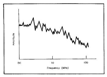
Fig 1—Spark-generated interference generally decreases in strength with rising frequency. The text describes how this characteristic can help you localize an interference source.
