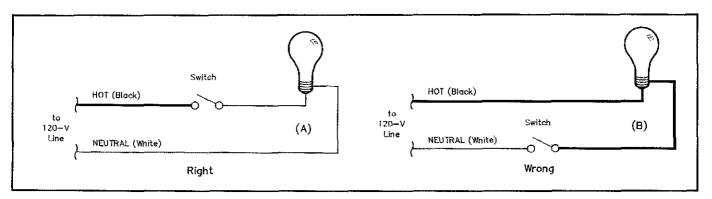
Fig 3—Correct light-switch wiring (A) interrupts the hot connection between the light fixture and the ac line. Incorrect wiring (B) leaves the fixture and much more of the wiring connected to the hot ac wire whether the switch is on or off. Turning the switch off in B cannot quiet line noise caused by hot-to-ground sparking in the light fixture.
