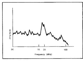
Fig 2—Spark-generated interference may not generally decrease in strength with rising frequency when power lines associated with the noise source resonate and peak the noise at one or more frequencies.
