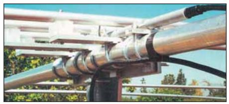
Figure 3—The area around the boom-to-mast plate for the KC6T beam. The Cal-Av Labs balun is mounted under the rearward 10 meter open-sleeve driver. All elements are mounted on the boom-to-element plates using cast acrylic-insulating blocks.
