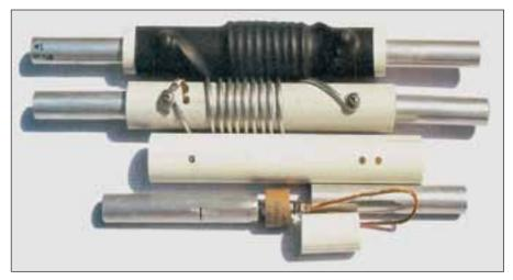
Figure 2—The trap assembly is shown in various stages of fabrication. The mechanical components are detailed in the drawing package available on the ARRLWeb site. This photo shows the 50 pF NPO capacitor attached to its trap terminal, complete with a flexible wire. The coil form and insert are also shown. Although this particular design used a shrink-sleeve cover, the final design used two coats of gray epoxy paint instead.
