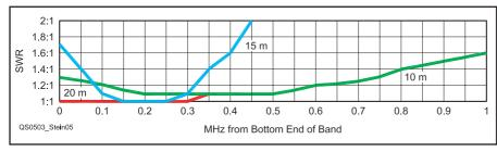
Figure 5—Measured SWR plots across the 10/15/20 meter bands at a height of 37 feet.
