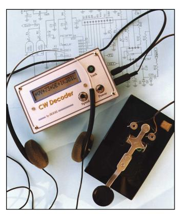
The asterisks appearing at the interword spaces are generated by sending a bogus Morse character. This display was generated using the straight key and as shown here, interword spacing is turned off.
