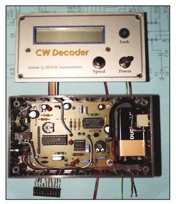
An inside view of the decoder. The LCD's 10-pin connector at the bottom-left in the photo attaches to the PC-board-mounted connector at the left near the PIC (U1) and pot (RV1).
