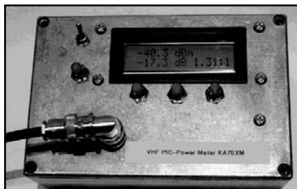
Fig 1—Exterior view of the PIC power meter.
