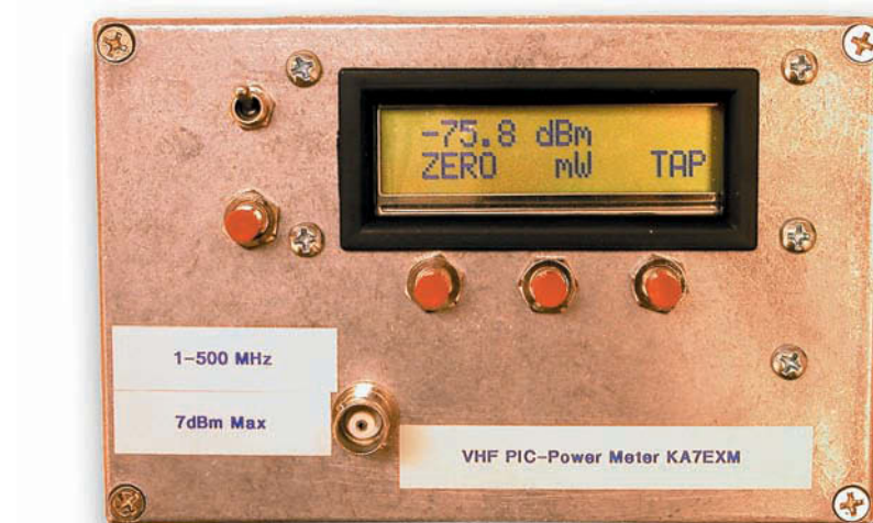
Figure 1—Exterior view of the PIC power meter.
