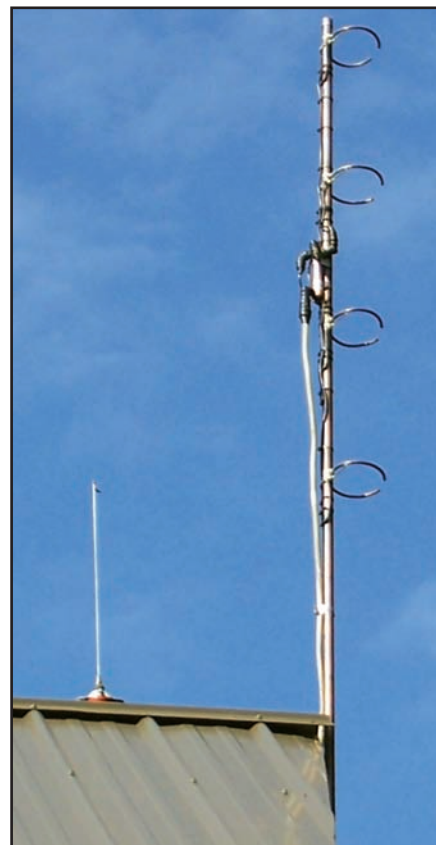
Figure 4 — Four Lowe's Loops mounted in a stacked array for additional horizontally polarized gain.
