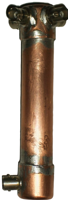
Figure 8 — Completed four way combiner/transformer assembly.
