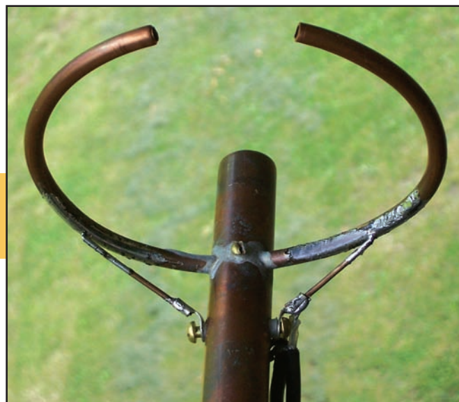
Figure 1 — Completed 432 MHz "Lowe's Loop."
