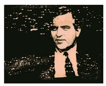
Figure 5—A typical electrical noise pattern as seen on a TV image.
