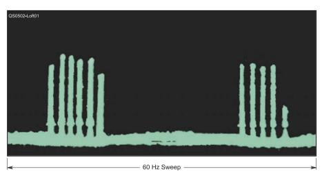
Figure 1—Power line noise pulses detected at 75 MHz, about 2 MHz below the NTSC channel 5 television video carrier.
