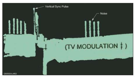
Figure 2—An NTSC channel 5 television video pattern, at the vertical rate (59.94 Hz). The noise pattern can be clearly seen.
