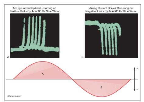
Figure 3—The relationship of the arcing current spike groups to the power line sine wave of 60 Hz.
