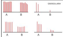
Figure 4—Examples of RF noise pulses, after detection by a TV field strength meter. The pulses will appear as spikes on each half-cycle of the power line ac waveform.
