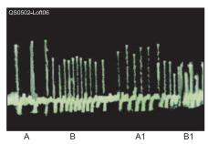
Figure 6-Two noise patterns, representative of two power line noise sources. Patterns A and A1 are both half-cycles of one pattern; B and B1 are of another
