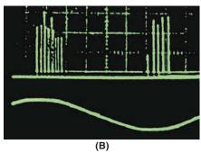
Figure 7-Noise patterns at 50 MHz and at 500 MHz, with a 60 Hz reference trace. Note that the pattern remains substantially the same in shape and format. The pattern at A is at 50 MHz. The pattern at B is at 500 MHz, with a 60 Hz reference trace. As one gets closer to a noise source, the pattern appears at higher frequencies.
