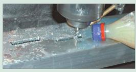
Figure A—The design of the slot antenna allows it to be easily reproduced with a milling machine.
