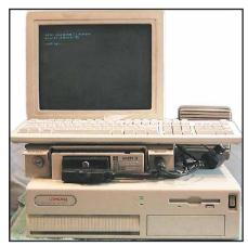
Figure 2—A typical node with a commercial link radio controlled by a PC. This is node 3350, Denver, Colorado. The link radio shown is a surplus GE Mastr II.
