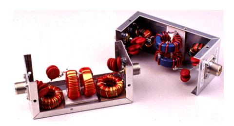
An inside view of 160 meter and 10 meter BPFs housed in  $2^{1}/_{4}\times 2^{1}/_{4}\times 5$ -inch (HWD) boxes equipped with SO-239 connectors at each end. With the exception of the 10 meter BPF, the filters are now housed in slightly larger boxes— $2^{1}/_{8}\times 3\times 5^{1}/_{4}$ -inch (HWD)—to lessen component crowding and minimize response degeneration when the cover is installed.
