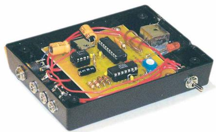
Figure 2—The prototype IR remote control receiver.
