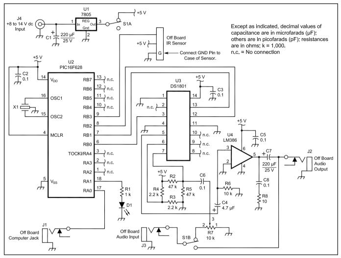
Figure 1—The IR remote control receiver schematic. All resistors are ¼ W, 5% tolerance. Parenthetical part numbers are RadioShack, www.radioshack.com/; all other parts as indicated. Digi-Key Corp, 701 Brooks Ave South, Thief River Falls, MN 56701; tel 800 344-4539; www.digikey.com/. Be sure to solder the ground pin to the IR sensor case, if not already done.
